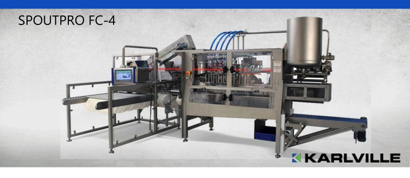
Pouch filling machine: SPOUT PRO-FC-4. Automatic pouch filling through the spout and capping machine.
