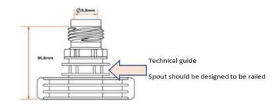
Filling through the spout (FTS) is the safest and most efficient method, allowing as little as 15mm head space below the spout.
