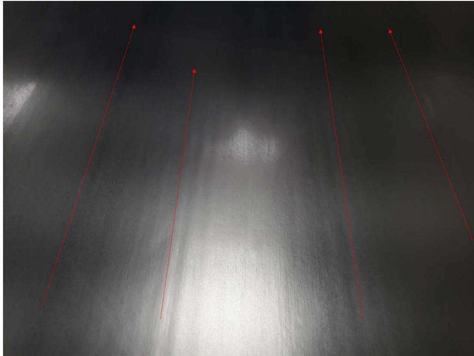
**Figure 2.** MET-BOPP (XR588) visual inspection showing non-uniform TAP coating
