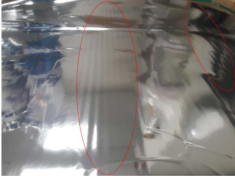
**Figure 1.** MET-BOPP (XR589) visual inspection showing wrinkles in film
