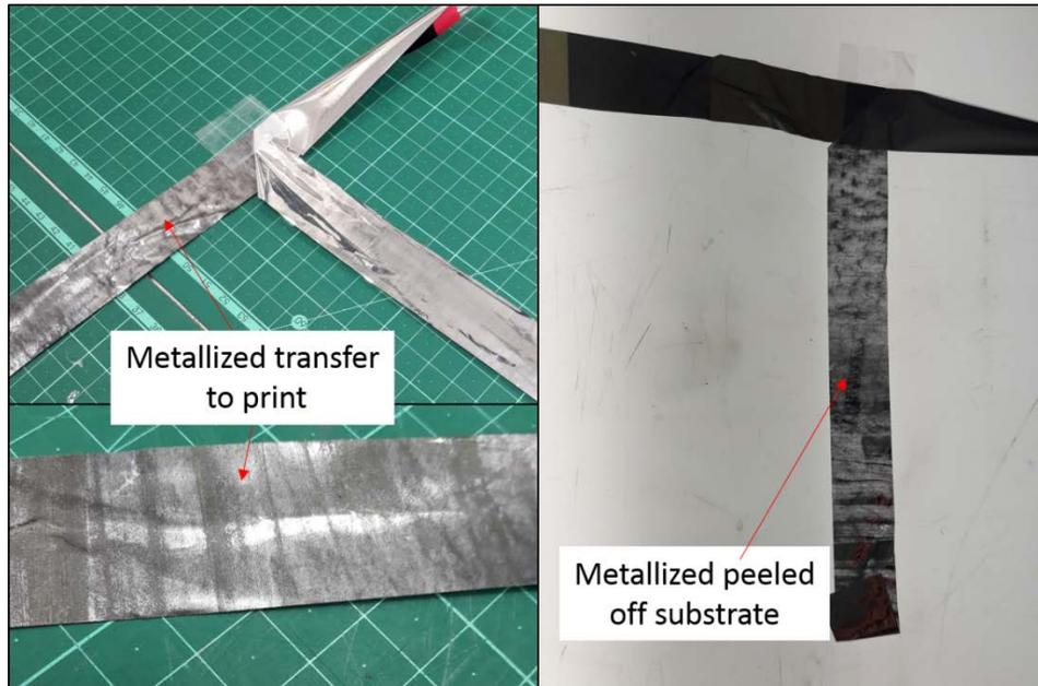
**Figure 5.** Visual inspection of delamination (left) and using back-light (right) showing the metallized layer failure
