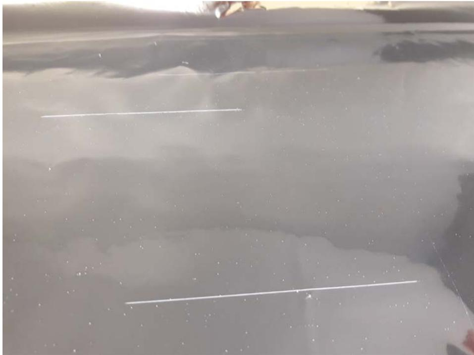
**Figure 3.** MET-BOPP (XR589) visual inspection of metallized layer (using back-light) showing holes and scratches in metallized layer
