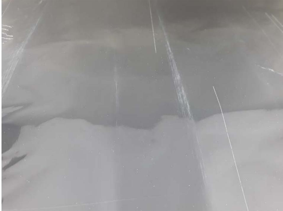
**Figure 4.** MET-BOPP (XR588) visual inspection of metallized layer (using back-light) showing holes and scratches in metallized layer
